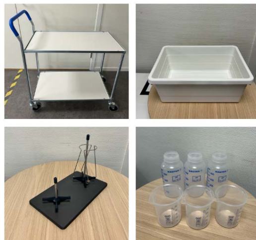
Fig. 2: All the teams received equipment to mock-up the lab automation use-case. The equipment included a cart with 4 castor wheels, a plastic bin, a plastic base hosting 2 different types of dishwasher pins (to mimic the dishwasher tray), 3 plastic bottles, and 3 plastic beakers.
