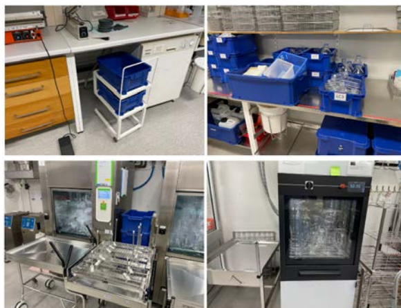
Fig. 1: Lab Automation use-case in the AstraZeneca chemical laboratories: a human operator drives a cart around the lab to collect dirty glassware, organizes it in a dishwasher tray, and finally inserts the tray in the dishwasher.
