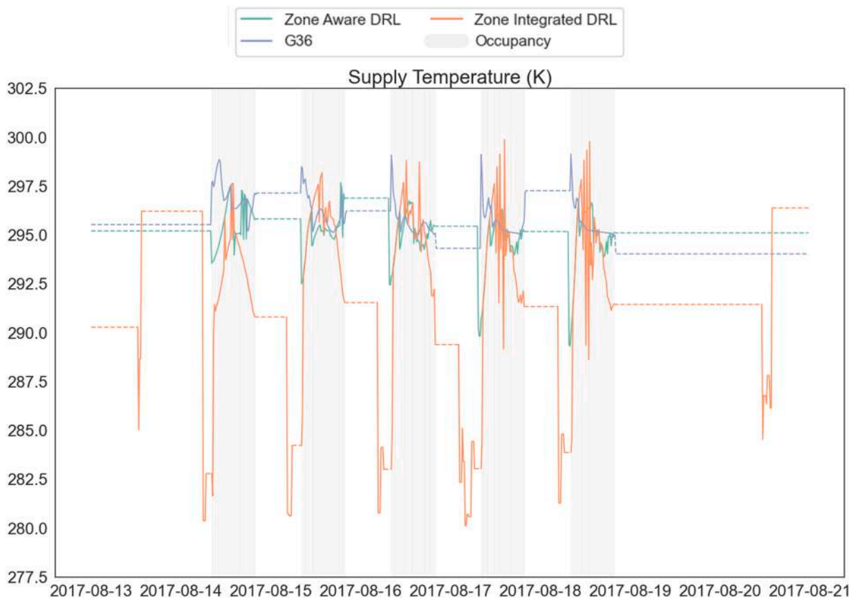
Fig. 18. Temporal pattern of supply temperature ( T_{sup} ) over a representative summer week for each control strategy (dashed lines indicate periods of system inactivity).
