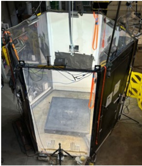
Fig. 1 Fragmentation cell developed at the University of Newcastle
