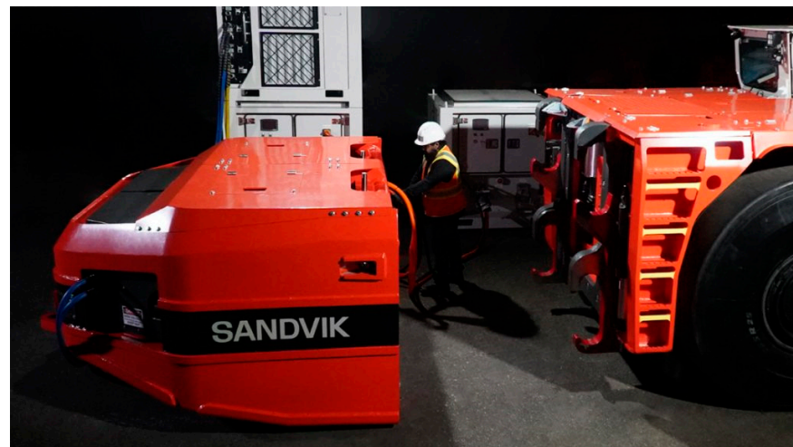
Figure 3. Lowered LHD battery and visible hooks on the machine (Company 2).
