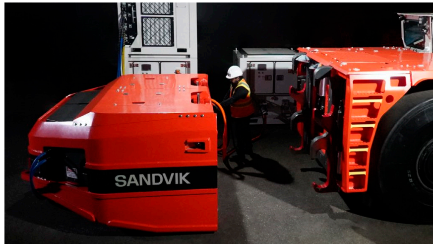
Figure 3. Lowered LHD battery and visible hooks on the machine (Company 2).
