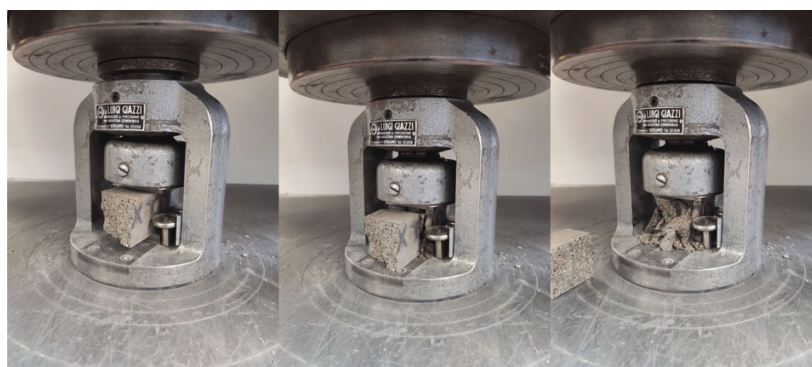
Figure 3. Compressive test of mortar specimens.
