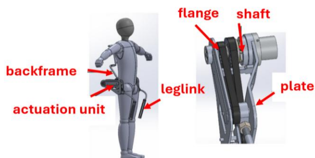
Figure 15a CAD model A and the exoskeleton with details of the actuation unit.
