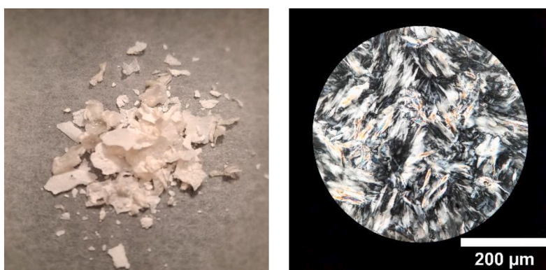
Fig. 8. Macroscopic appearance of extracted wax (Left); PLM images of re-crystallized RBX obtained with Process #2 (Right).
