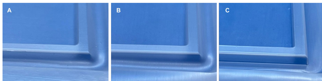
Figure 5. Representative pictures of a detail of the thermoformed trays obtained using (A) PLA + T_C-screw, (B) PLA + T_R-screw, and (C) PLA + T_B-screw.
