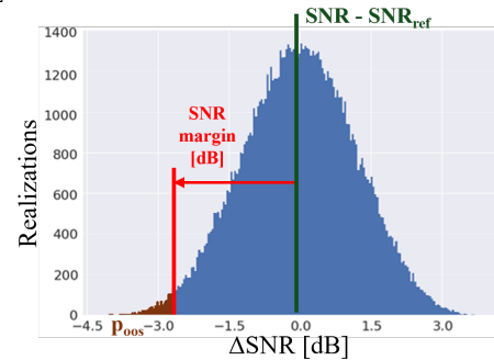
Fig. 5: System margin assessment on SNR distribution based on the maximum out of service probability P_{00s} .
