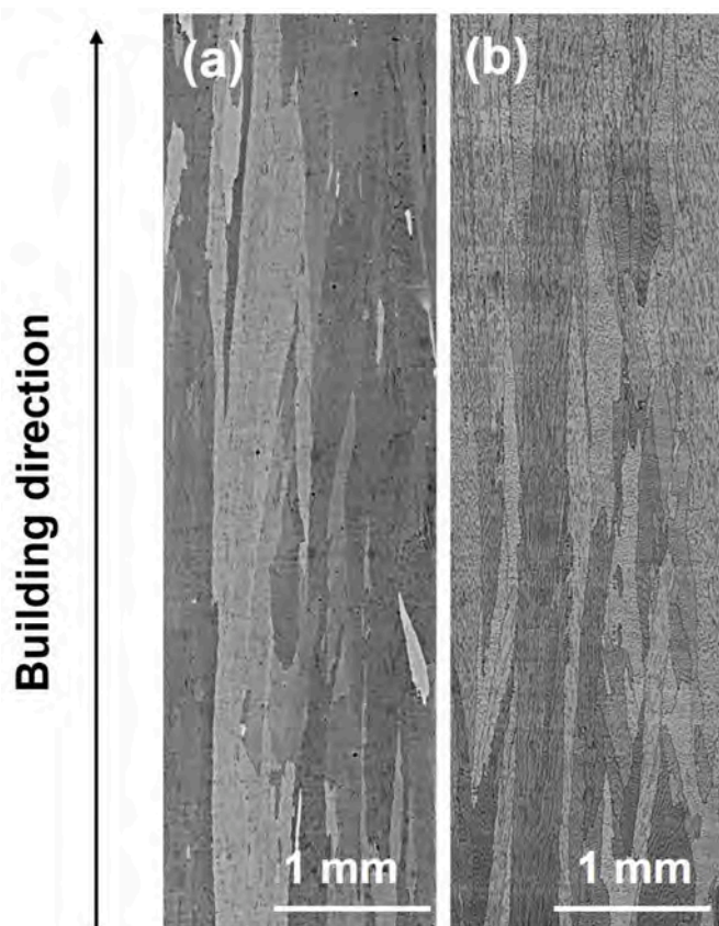
Fig. 4. Cross-section LOM images acquired along the building direction of a chemical etched (a) R1 and (b) R2 samples.
