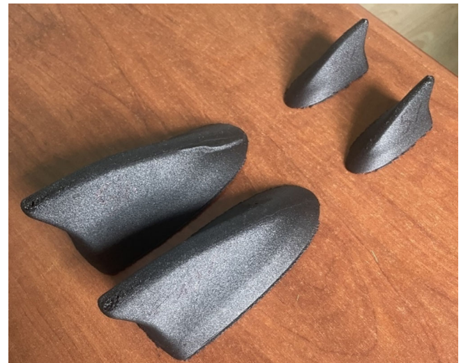
FIGURE 7 Three-dimensionally printed shark fin antenna covers using polyamide (PA)-recycled milled carbon fiber (rCF) filaments.
