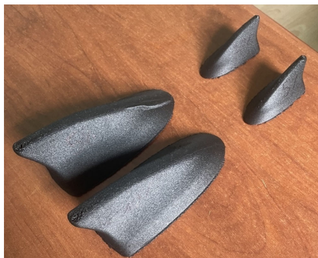
FIGURE 7 Three-dimensionally printed shark fin antenna covers using polyamide (PA)-recycled milled carbon fiber (rCF) filaments.
