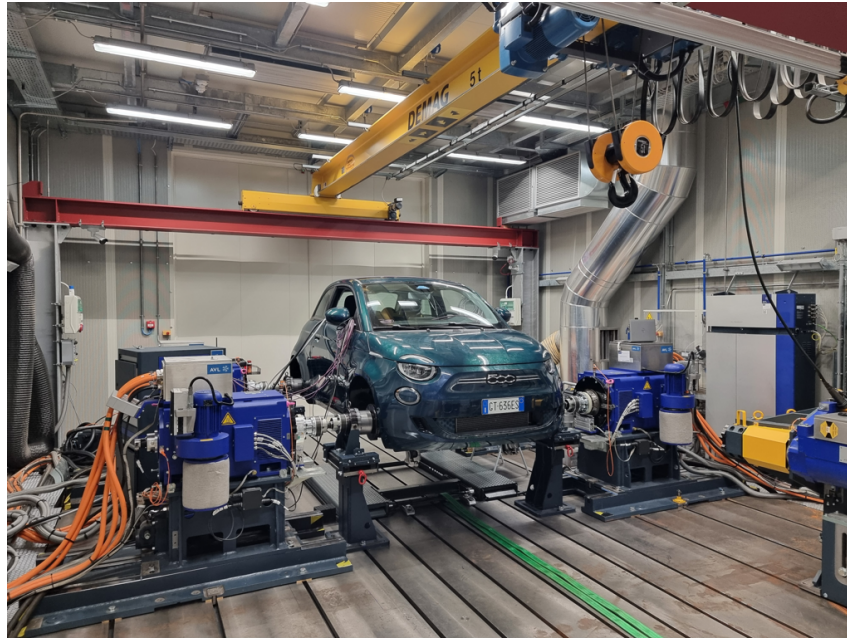
Fig. 2.31 Fiat 500e donor vehicle characterization in CARS@Polito test bench.
