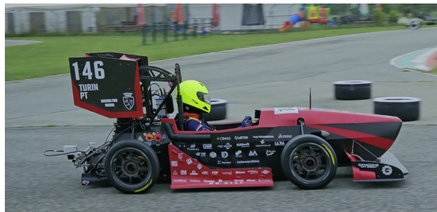
Fig. 4.13 Squadra Corse Polito 2024 prototype during track testing session. Ground speed sensor installed on the rear of the vehicle.
