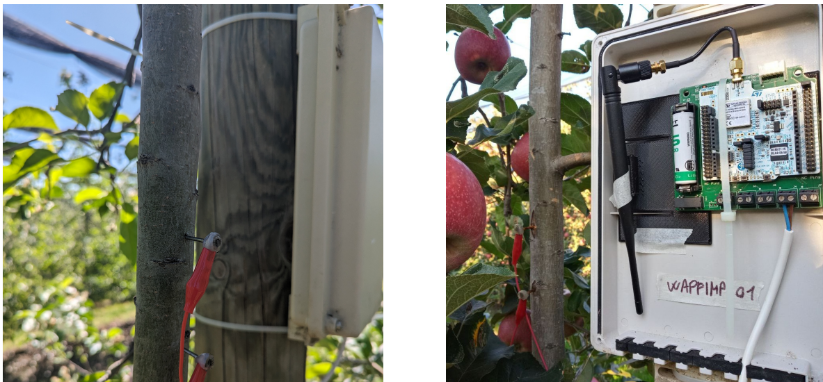
Figure 2: Stem frequency sensor installed in F1 farmer where the electrode distance is 5 cm. Exactly the same configuration has been used, except for an electrode distance of 15 cm in the two sites of F2 farmer. (Left) Zoom on electrodes connected in the stem of the apple orchard. (Right) Zoom on WAPPIMP stem frequency sensor board in the field.
