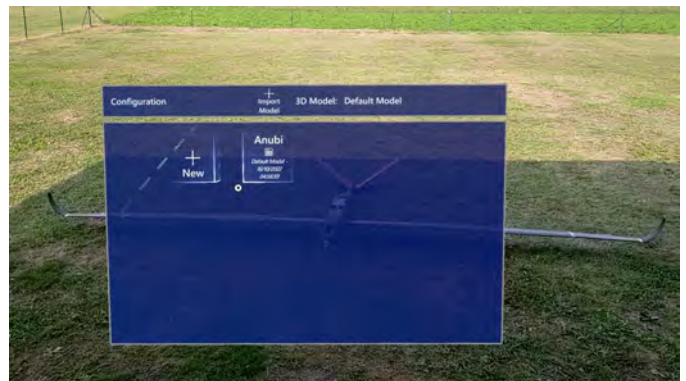
Fig. 2. A picture showing the Selection phase of the PhotoNext FBG AR Viewer software. The "Import Model" located at the top of the window allows the import of a new model, while the "New" button allows the creation of a new sensors configuration. Any other buttons created right or below it are relative to any previously created sensors configurations.
