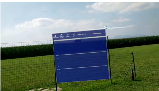
Fig. 4. A picture showing the Monitoring phase of the PhotoNext FBG AR Viewer software during the tests carried out. The buttons at the top of the window allow to hide or show both views, fix the window, and close the software.
