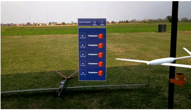
Fig. 3. A picture showing the Configuration phase of the PhotoNext FBG AR Viewer software. The "Save" and "Start" buttons located on the top of the window allow the current sensors configuration to be saved and the Monitoring phase to start. The central part of the windows allows to view the detected sensors to change their respective type and position them on the chosen model.
