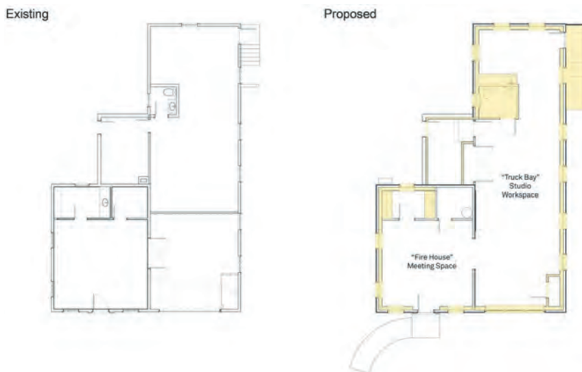
Figure 2. Plans of the Phoenix as existing and proposed showing added in yellow - 2x4 stud wall, insulation, new windows, kitchenette and accessible restroom.
