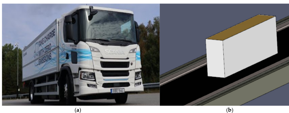
Figure 3. (a) Image of the SCANIA 25 P BEV; (b) its representation in PyroSim.
