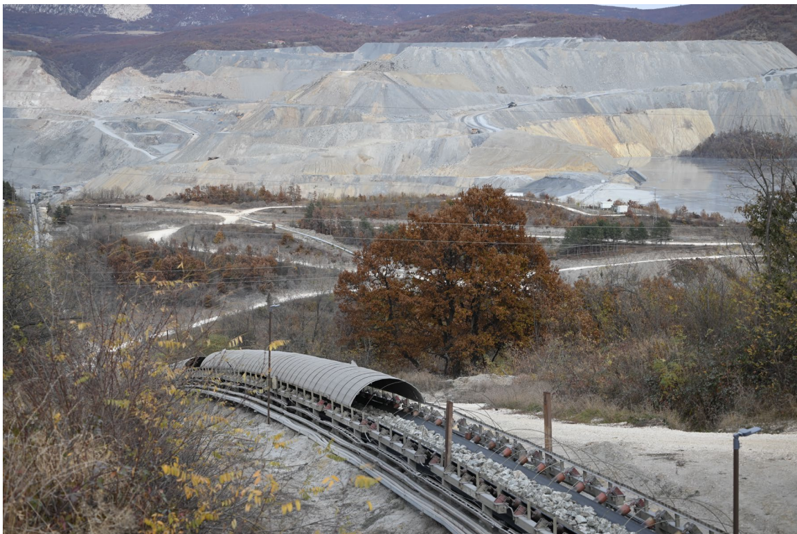
Figure 1. Operational landscape of mining infrastructure illustrating the extended spatial footprint of resource extraction. This photograph depicts a conveyor belt transporting overburden—the approximately 99% waste material resulting from copper mining activities—from the Veliki Krivelj open-pit mine toward a dumping site located over 10 km away near Bor, Serbia. The extensive
