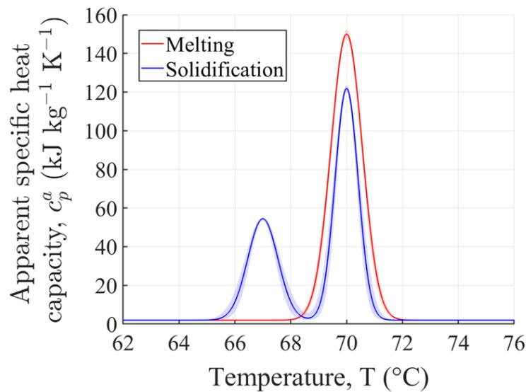
**Figure 3.** Apparent specific heat capacity of the investigated PCM, with shaded regions indicating the uncertainty in the fitted curves based on the data provided in Table 1. The figure is adapted from ref. [22].
