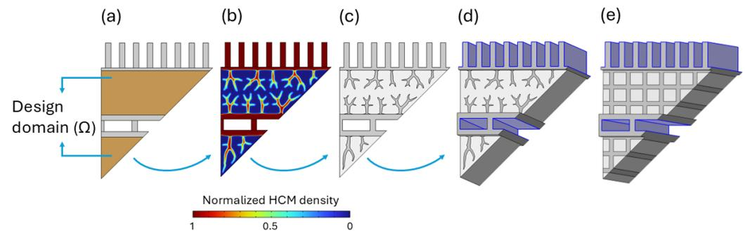
**Figure 2.** Evolution of the topology optimization design: (a) Initial guess of the design, (b) Output material volume factor ( $\theta$ ), (c) Final 2D geometry, and (d) Extruded 3D geometry including simulation domains. The simplified reference geometry is shown in (e). To reduce computational cost, geometric symmetries were exploited, and only one-eighth of the device was simulated.
