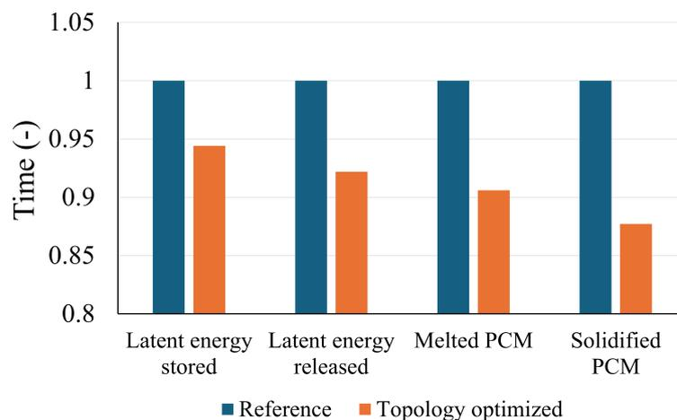
**Figure 5.** Time to store or release 90% of the latent energy and achieve 90% melting or solidification of the PCM. The vertical axis is normalized by the corresponding  $t_{90}$  value of the reference case.
