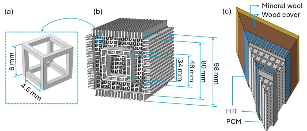
**Figure 1.** Design of the LHTES mock-up (from Morciano et al. [22]): (a) Unit cell of the Cartesian lattice, (b) 3D CAD model of the device, and (c) 3D computational model illustrating the simulation domains. To reduce computational cost, geometric symmetries were exploited, and only one-eighth of the device was simulated.
