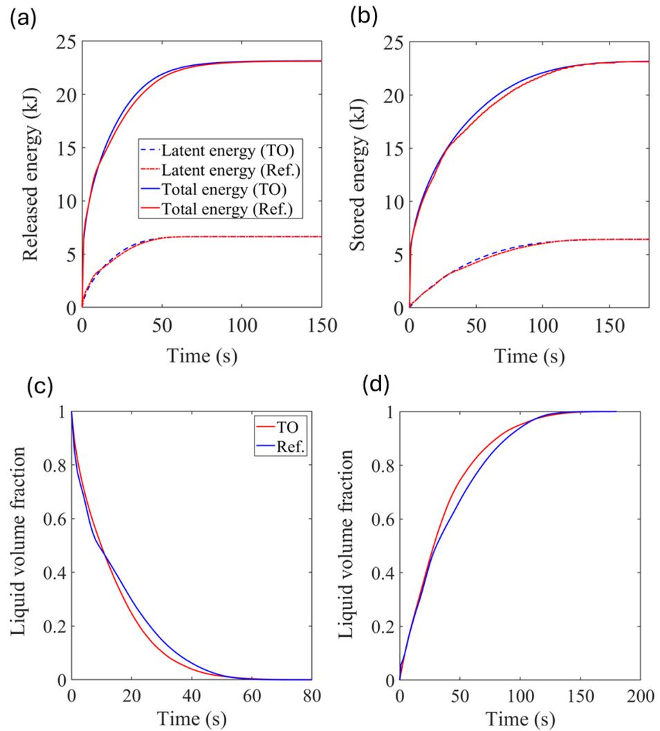
**Figure 4.** Performance comparison between the simplified reference model and the topology-optimized (TO) model: (a) Thermal energy released, (b) Thermal energy stored and liquid volume fraction of the PCM during (c) discharging and (d) charging.
