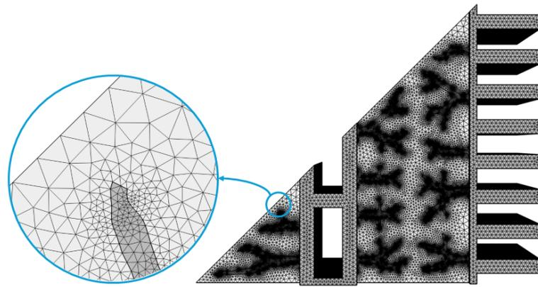
**Figure A2.** A view of the chosen computational grid.
