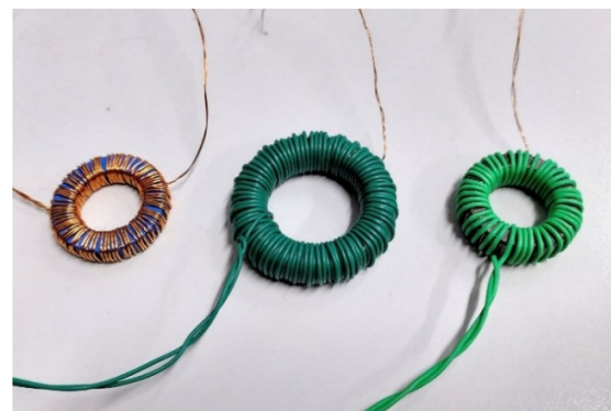
Fig. 7. The three measured toroidal samples (laminated, SMC, amorphous)
