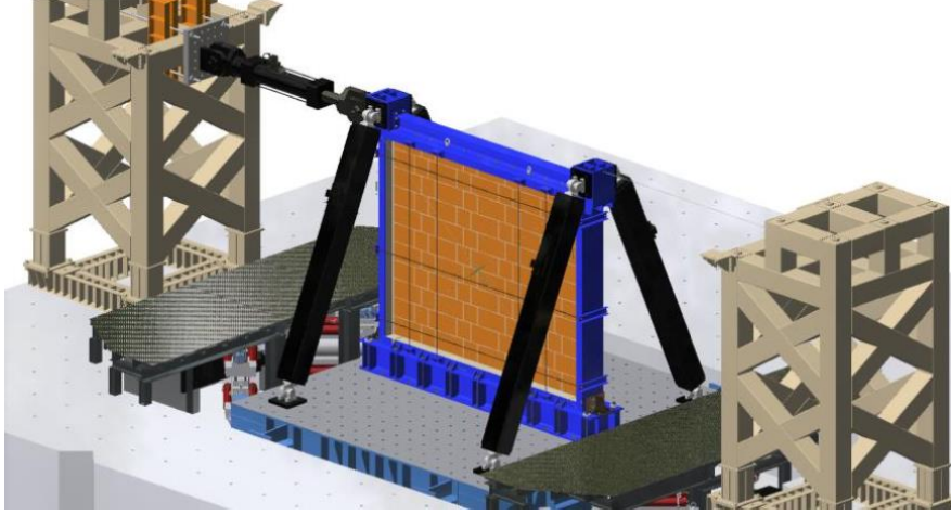
Fig. 3. Sketch of the experimental setup adopted for the quasi-static IP and dynamic OOP tests (Kurukulasuriya et al., 2023).
