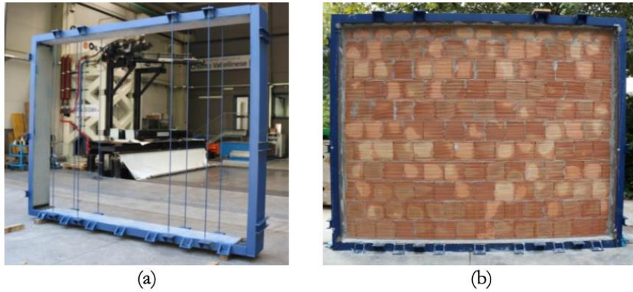
Fig. 2. (a) Structural frame; (b) masonry infill at the end of the construction (Kurukulasuriya et al., 2023).
