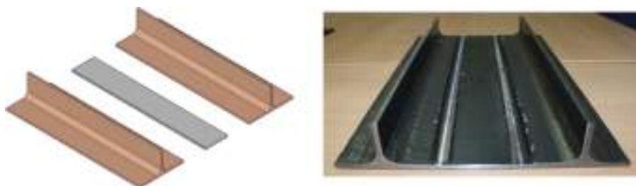
Fig. 1. Integrally Stiffened Plate demonstration fabricated by friction stir butt welding two rolled T sections to a steel plate. Source: Authors.
