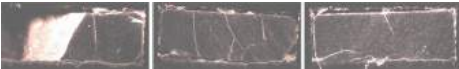
Fig. 5. Image of PM cross-section from the side for top layer printing powers 220 W (left), 200 W (middle), 180 W (right). Source: Authors.
