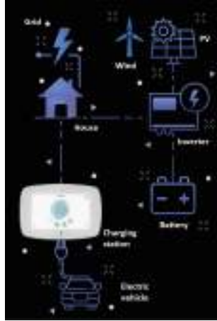
Fig. 1. Topology of the PV/wind grid-connected electric vehicle charging scheme
