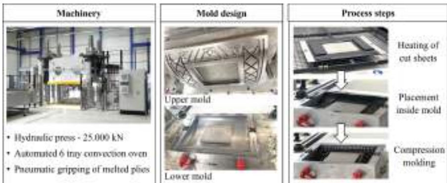
Fig. 4. Manufacturing setup. Left: hydraulic press; middle: upper and lower halves of the two-piece mold; right: basic processing steps of the compression molding process. Image courtesy of CG Rail GmbH, reproduced with permission.
