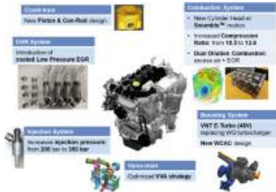
Fig. 2. Features and Modifications of the PHOENICE Engine Compared to the Baseline [5]
