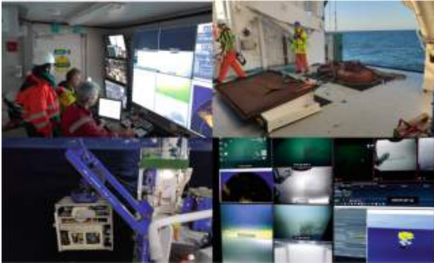
Fig. 2. Use of an ROV at sea to undertake scanning of an area of a ship to be repaired. Source: Authors.
