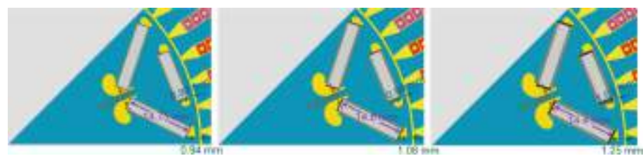
Fig. 3. Designs with 0.15 mm (left), 0.3 mm (middle), and 0.5 mm (right) thick encapsulations.
