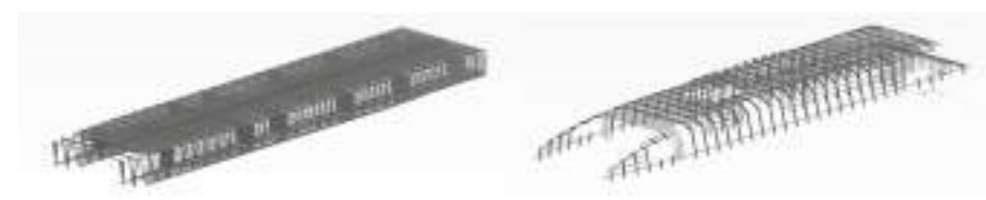
Fig. 4. Parametric Structural Models for Hull and Superstructure Weight Estimation (Source: Authors)
