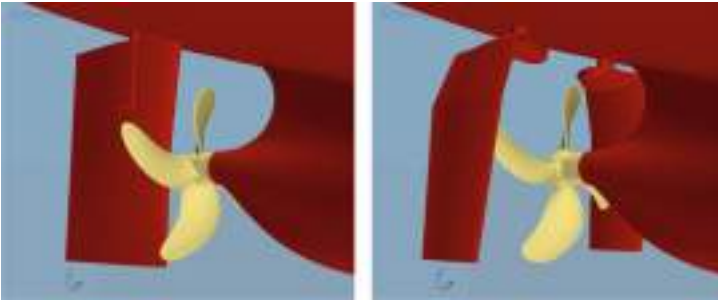
Fig. 5. Conventional FPP and rudder (left), CPP with Gate-Rudder (right) (source: authors)
