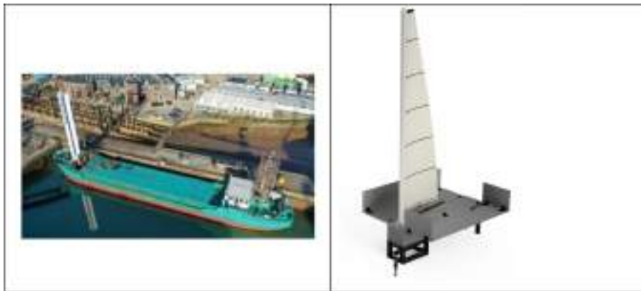
Fig. 2. Left: Rigid eSAIL® system - Reproduced with permission from Bound4Blue, copyright Bound4Blue, 2024; Right: sketches of the Semi Rigid Wing installation (Reproduced with permission from Advanced Wing Systems, copyright AWS, 2024).
