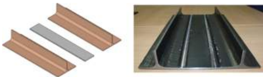
Fig. 1. Integrally Stiffened Plate demonstration fabricated by friction stir butt welding two rolled T sections to a steel plate. Source: Authors.
