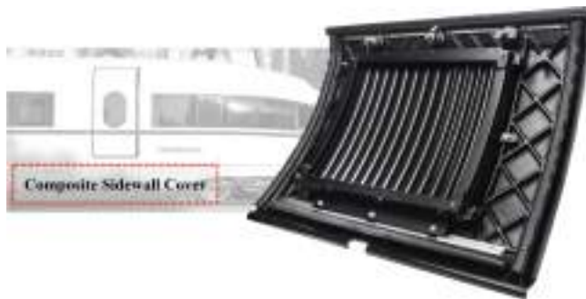
Fig. 5. Fully assembled lightweight component [6]
