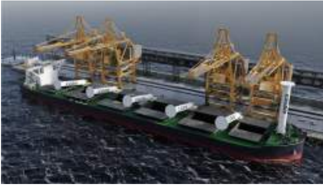
Fig. 4. Proposed deck layout for the new-build concept vessel (source: authors, image produced using Adobe Suite and Blender)
