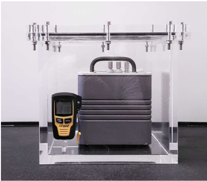
Fig. 6. Airtight container employed to perform the cooling event described in Section III, Fig. 4(b) to avoid possible humidity condensation effects. The yellow instrument is the environmental parameter data logger.
