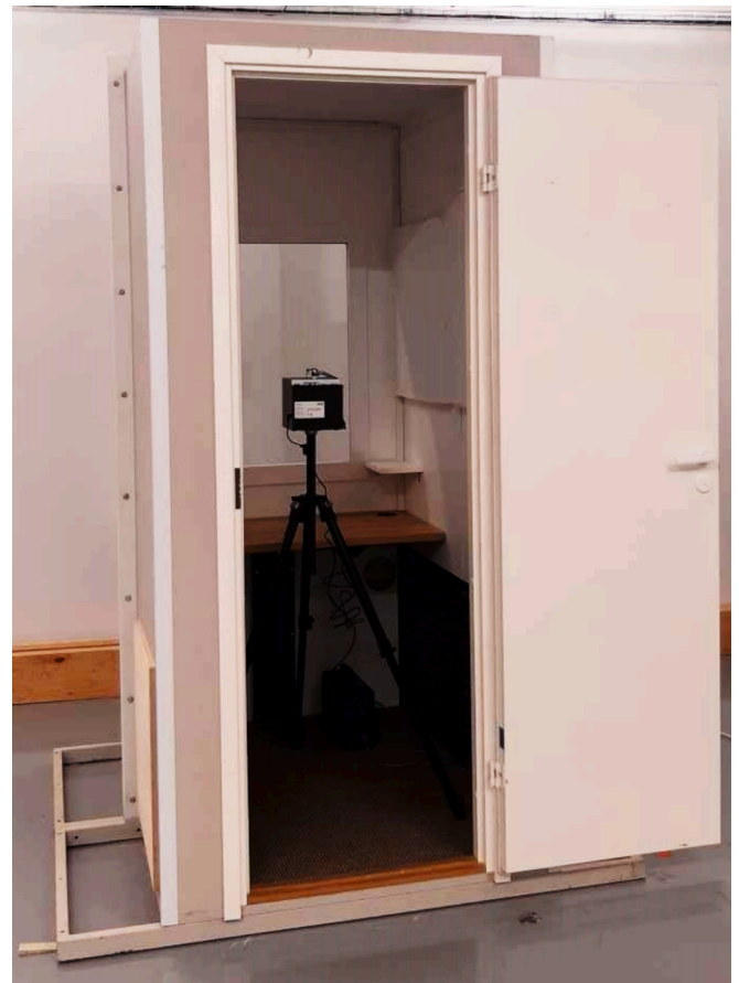
Fig. 1. The booth used in the between-laboratory experiment. The outer dimensions were 1.05 \times 1.41 \times 2.25 m. The photograph represents Object 1 (booth with door 180° open) under the Scenario 2 test where the artificial mouth inside the object and pointing towards the sitting occupant's direction.
