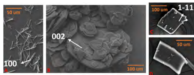
Figure 12. SEM images of (A) QDH, (B) QDMSO, and (C, D) Que-Im crystals. Facet orientations are depicted with white labels and arrows.
