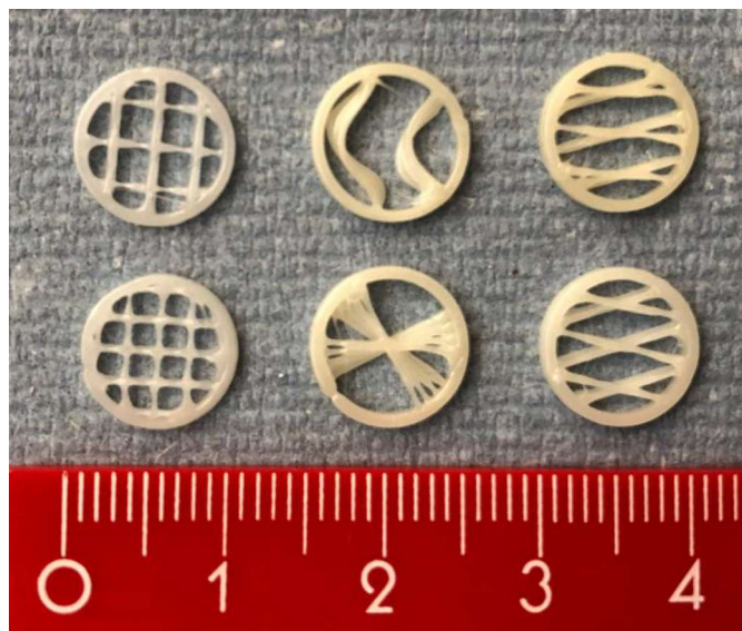
Fig. 1: Multi-layered structures with different patterns fabricated by melt extrusion additive manufacturing.
