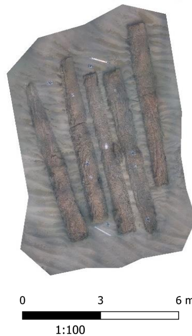
Figure 16. Final orthophoto derived from the 3D model of the five columns.
