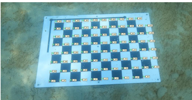
Figure 8. The calibration panel on the seabed with the 88 markers detected by the Agisoft Metashape software.
