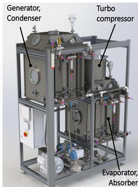
Figure 1: Design of the lab-scale hybrid chiller (Schweigler, 2019).
