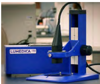
(a) Picture of the budget OCT used in this work (credit: Lumedica [23]).
