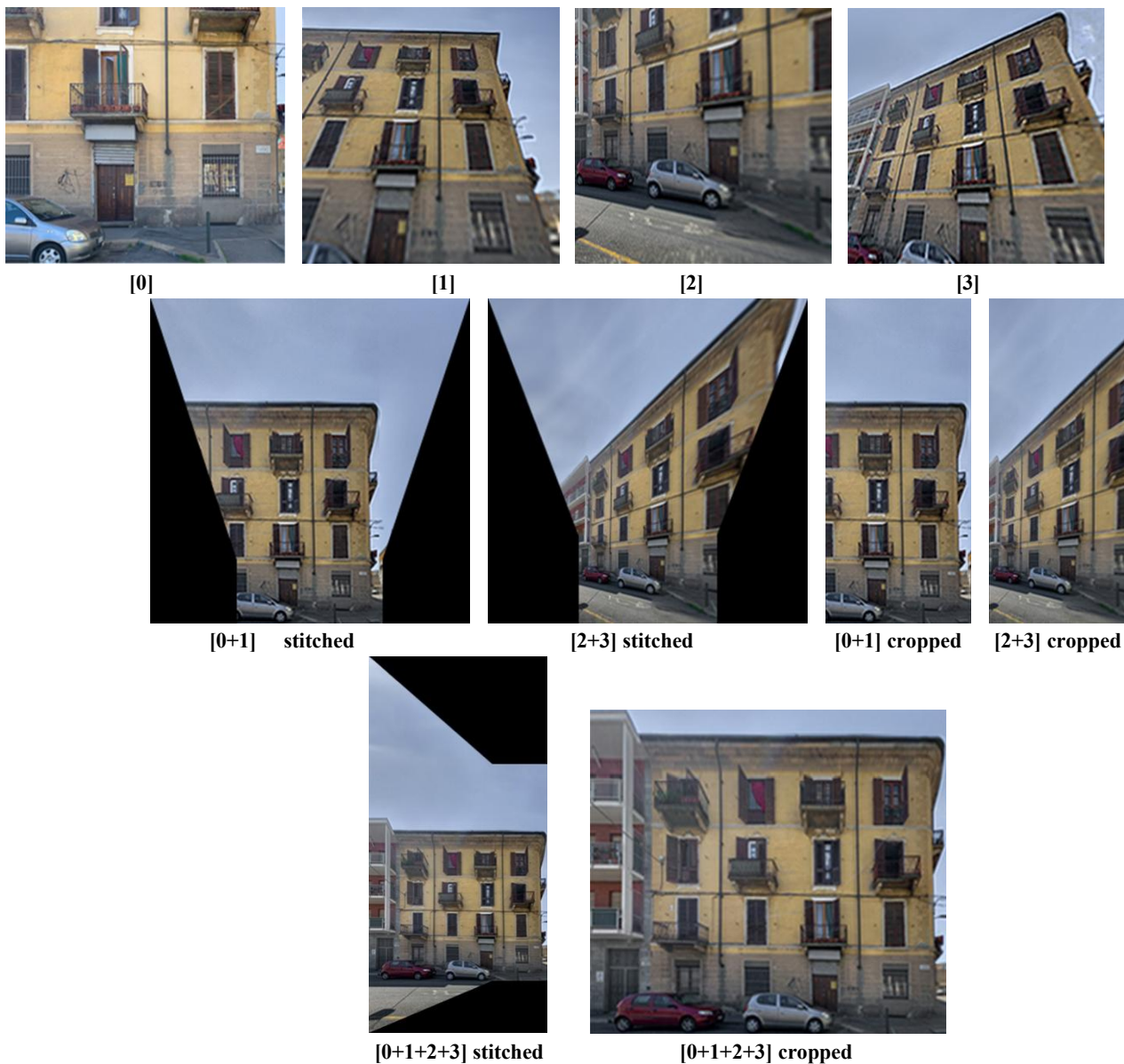
Figure 5. Automatic image extraction, cropping, and stitching. Top row: original images 0, 1, 2, and 3. Middle row: first round of stitching/cropping. Bottom row: second (final) round of stitching/cropping.
