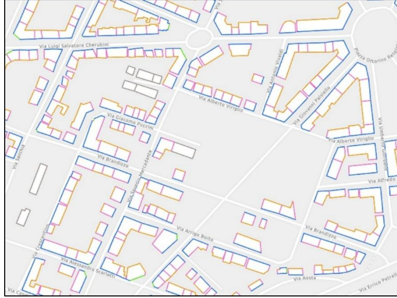
Figure 12. Visualization of automatic building classification. Street-facing façades as identified during GIS stage are shown in blue. Classification algorithm output: green = additional street-facing façade; magenta = non-street-facing side; orange = rear. Buildings not classified (gray) are in the OSM database but had no street-facing front identified at GIS stage. Basemap source: Esri (2024).
