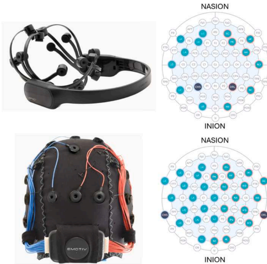
Fig. 3. 14-channel EEG headset (above, left) and its electrode position (above, right); 32-channel EEG head cap (below, left) and its electrode position (below, right).
