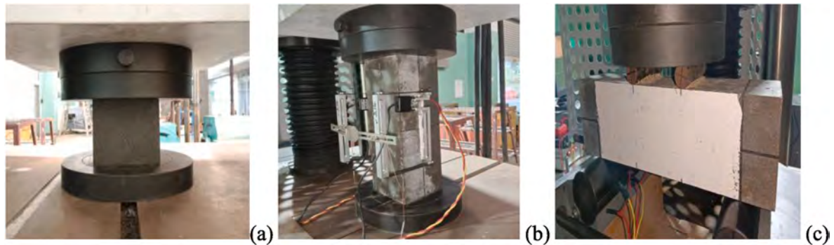
Fig. 6. Preliminary tests of UHPC: Compression (a), (b); Bending (c).
