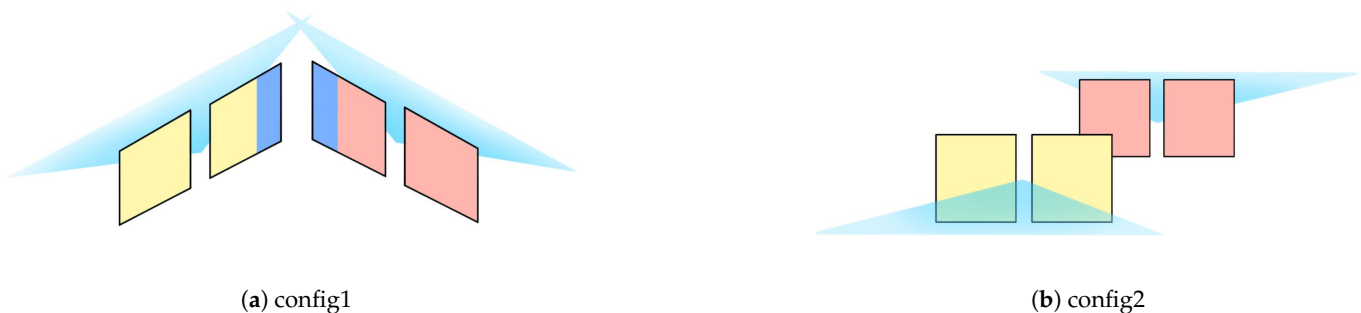
Figure 4. Stereo camera configurations: (a) Stereo 1 (cam0 and cam1, yellow field of view) and Stereo 2 (cam2 and cam3, red field of view) with shared field of view between cam1 and cam2 (blue); (b) Stereo 1 and Stereo 2 with non-overlapping fields of view.
