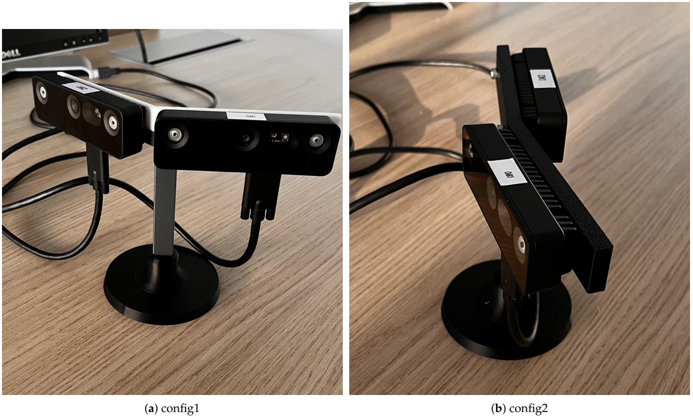
Figure 3. The two configurations of the multi-camera setup: (a) The two stereo cameras have a relative angle of 45 degrees; (b) The two stereo cameras point in different directions.
