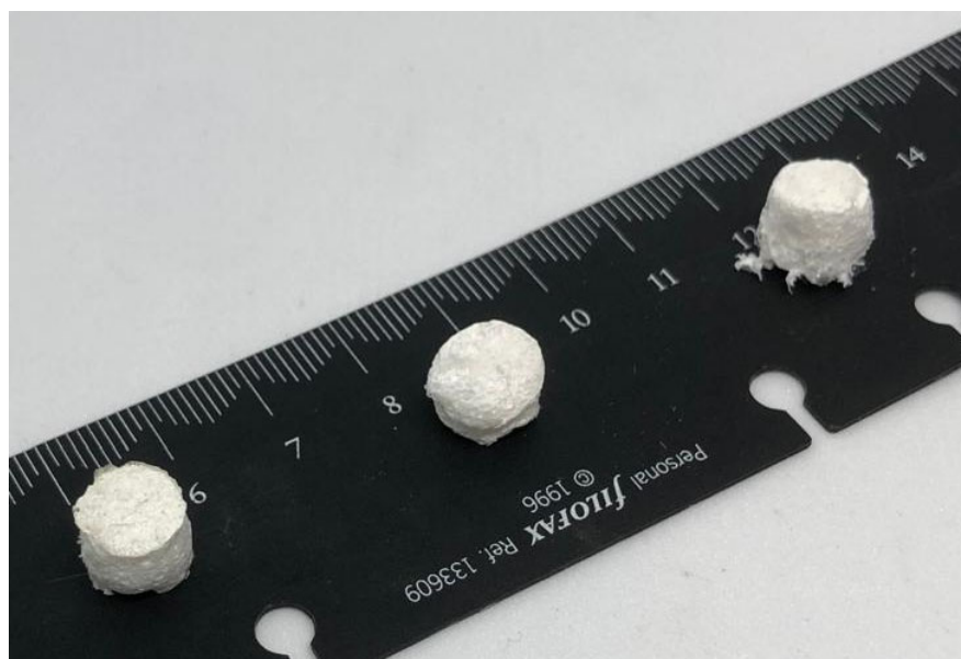
Figure 1. Hydrogels obtained after lyophilisation containing different concentrations of BG-Te-Sil bioactive glass and photocured. From left to right: MCHIT, MCHIT3, and MCHIT5.
