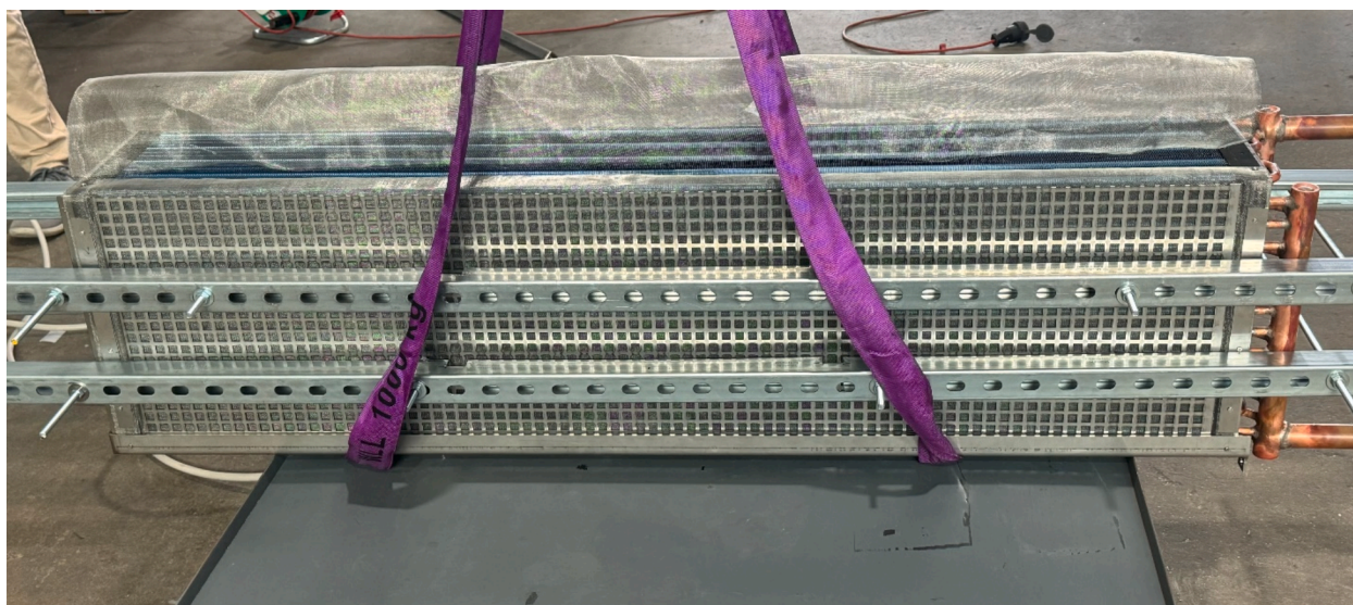
Fig. 6. Detail of the adsorbent, including the heat exchanger, 38 kg of sorbent and a surrounding structure able to keep the material inside.
