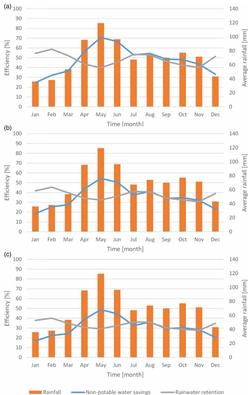
Figure 10 | Monthly variability of the efficiency of the RWH system associated with a traditional roof for building types 1 (a), 2 (b) and 3 (c) (tank capacity = 5 m 3 ).
