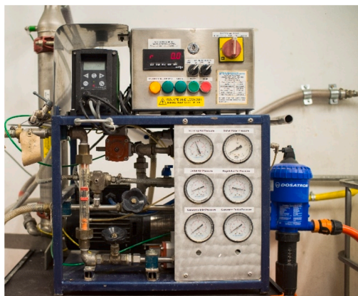
Fig. 4. Left: Foam generator picture. Right: Foam generator scheme. The generator operates with a maximum liquid flow of 11.9 l/min and a maximum air pressure of 4 bar, with both flow rates finely regulated through needle valves. The static mixer with specific dimensions, including an internal diameter ( D_i ) of 78 mm, a length ( L ) of 450 mm, and it is filled with glass fragments with a mean diameter of 5 mm. The volumetric pump for surfactant is equipped with a mixing chamber to ensure a correct mixing of water and surfactant.
