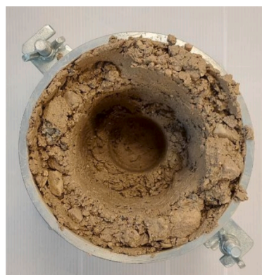
Fig. 5. Scheme of the soil flow under the blow of the Proctor ramming weight (left); Instance of failure of the Proctor test (right).
