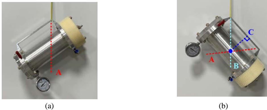
Figure 4-9 Determination of the gravity center of the GIS model by suspension method. (a) First record. (b) Second record.
