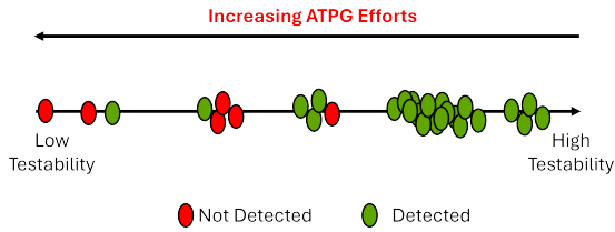
Fig. 1: ATPG Testability oriented fault detection capabilities vs. Test pattern generation efforts.
