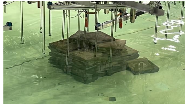
Figure 1 - Experimental setup employed to simulate the wave source survey inside the Aalborg University wave basin facility.
