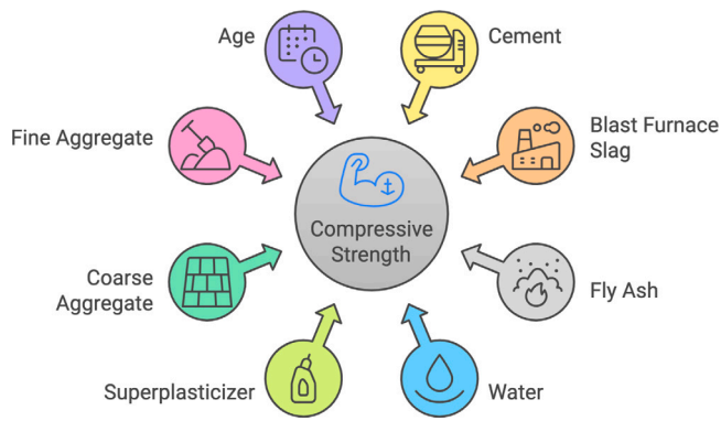
Fig. 1. Feature space for concrete compressive strength prediction.
