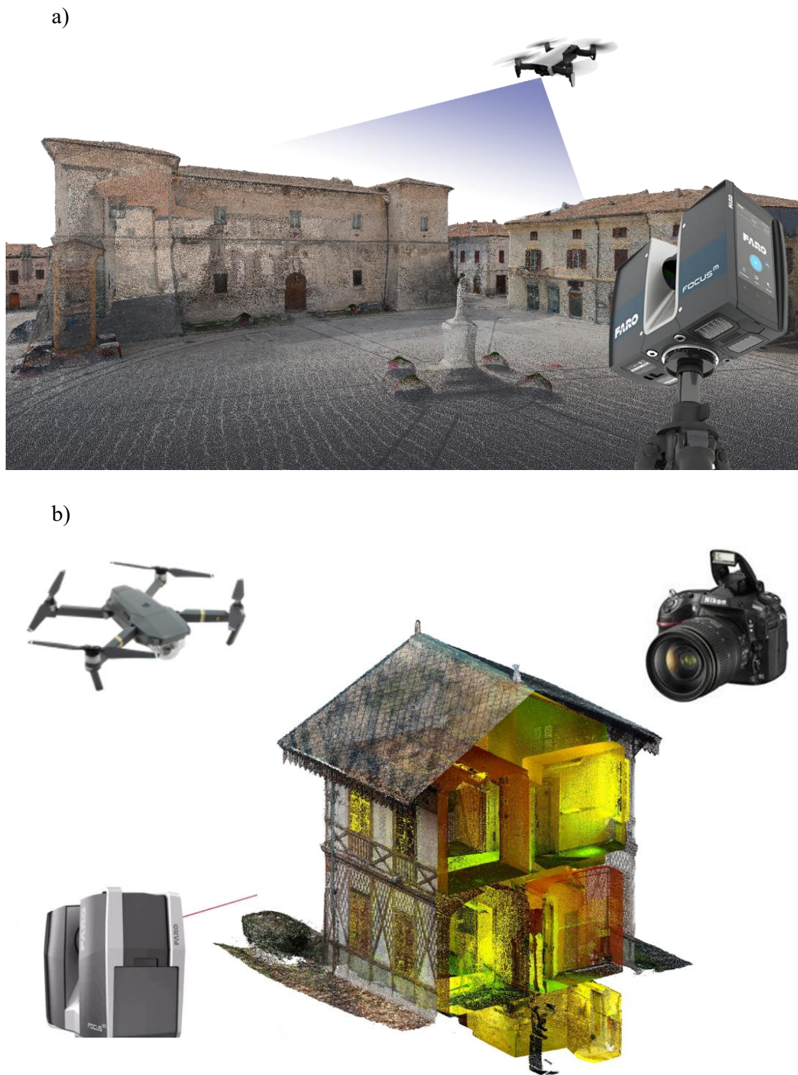
Figure 2_5: (a) Image depicting the point cloud of Piazza S. Benedetto in Norcia acquired by the integration of TLS and UAV techniques (Avena 2020); (b) Example of integrated 3D metric survey (TLS, UAV and terrestrial cameras techniques) of Villino Caprifoglio, Turin (Sammartano & Avena 2024).
