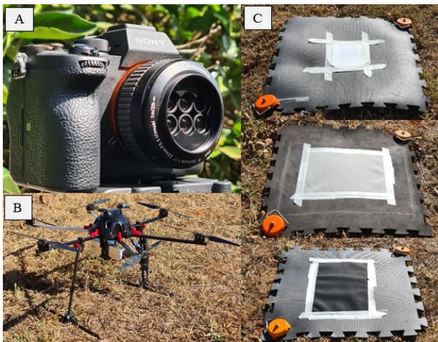
Figure 4. Aerial multispectral data collection. In (A) the AgroWing camera with six optical lens heads, in (B) the unmanned aerial vehicle, and in (C) the targets fixed in the field to carry out the empirical line calibration.
