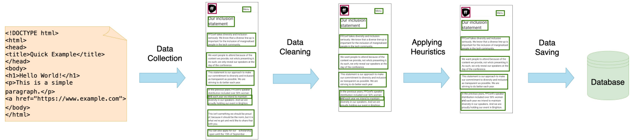
Figure 1: Overview of our pipeline, with its four stages: (i) data collection in which a headless browser is deployed in a given viewport and the UI is converted into a Figma-compatible JSON format, (ii) data cleaning in which non-visible elements and irrelevant attributes are removed, (iii) application of heuristics in which we apply domain-specific rules to filter duplicate, overlapping, or small elements to enhance dataset quality, and (iv) saving. For illustrative purposes, each stage is graphically represented by the picture obtained by applying the JSON content of the stage on the reference web-page screenshot.
