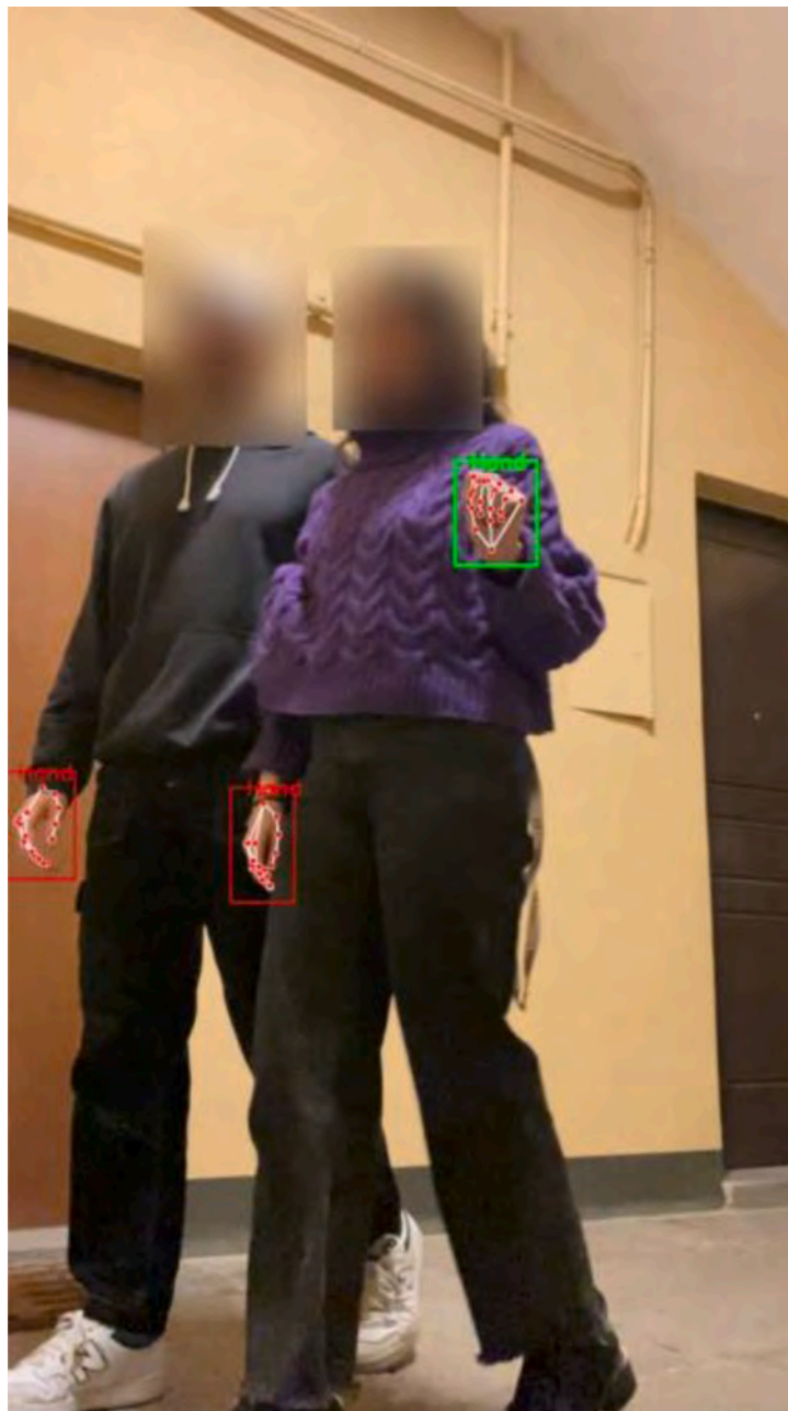
Fig. 8. Visualization of the Green Bounding Box Highlighting the Detected Signal and Face Blurring for Enhanced Privacy Protection.
