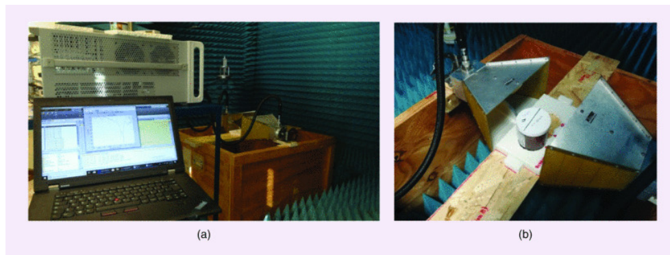
Figure 1.3.9: System configuration for simulating movement [65]: (a) the whole setup and (b) the two antennas positioned near the jar.
