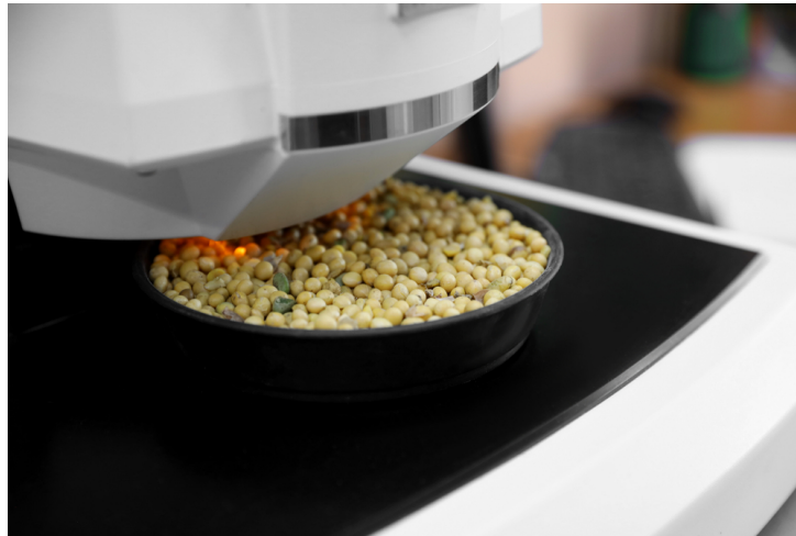
Figure 1.2.4: NIR imaging system in operation on a batch of olives [28].
