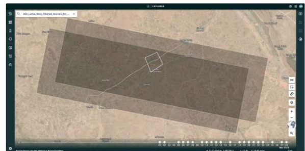
Figure 2. Footprint of stereopair-1 Images in Planet explorer over the studied area (in white rectangle).
