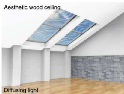
Figure 6: Comparing light diffusion through an aesthetic wood glazing with that through a standard glass ceiling. Adapted from Mi et al., 2020 under CC-BY licence
