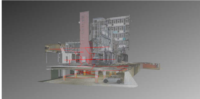
Figure 6. Acquisition path followed by the HMLS (in red) overlaid on the TLS point cloud.
