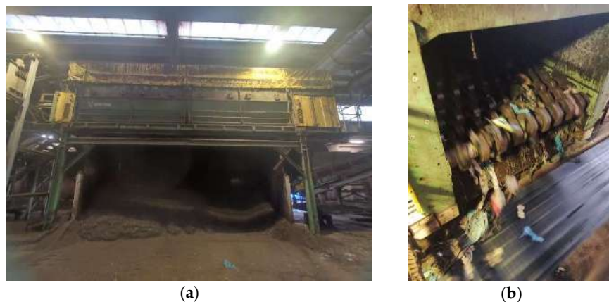
Figure 1. (a) The trommel screen and final compost (<12 mm) falling through, and (b) the disc screen (50 mm opening).
