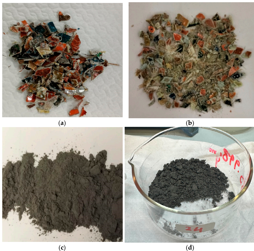
Figure 2. Images of the solvent-pretreated PCB samples: (a) Group 2 with particle size between 5.6 mm and 2 mm before solvent pretreatment; (b) Group 2 with particle size between 5.6 mm and 2 mm after solvent pretreatment; (c) Group 3 with particle size less than 400 \mu\text{m} before solvent pretreatment; and (d) Group 3 with particle size less than 400 \mu\text{m} after solvent pretreatment.
